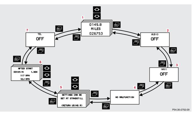
Depending on your vehicle's equipment, you may use the buttons on the multifunction steering wheel to call up, control and set the following systems in the multifunction display:
